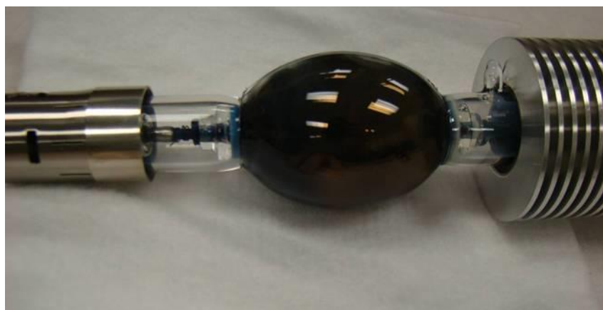
Figure 31: Lamp run under reverse polarity.
