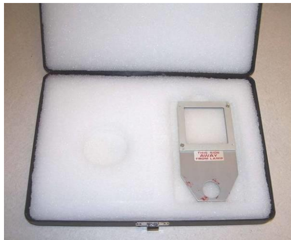
Figure 3: Air mass filter assembly (stored in case)
