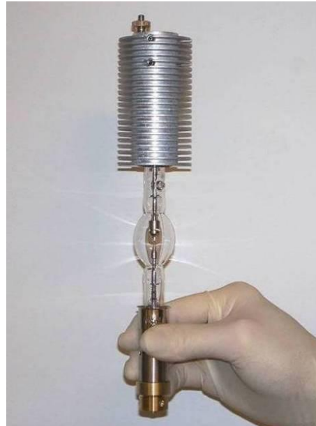
Figure 13: 450W Lamp with heat sink attached
