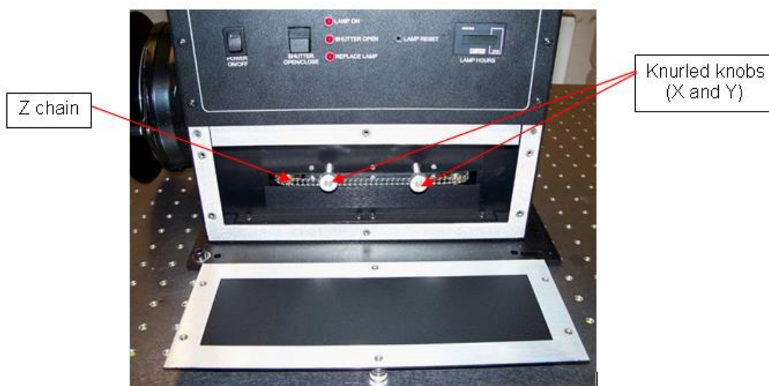
Figure 28: Lamp focus adjustment mechanisms (Access panel removed)
