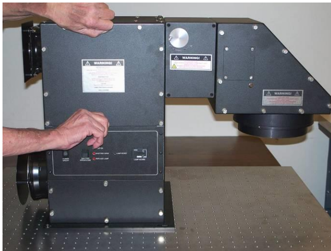
Figure 22: Removing the lamp access panel.
