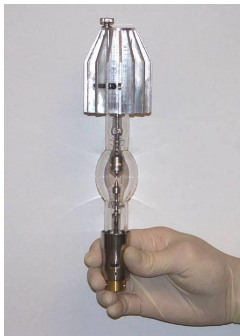
Figure 15: 1kW lamp with heat sink attached
