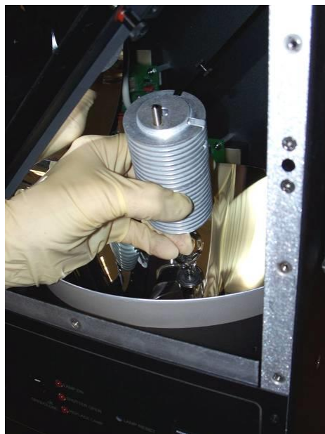
Figure 26: Heat sink unscrewed from socket.
