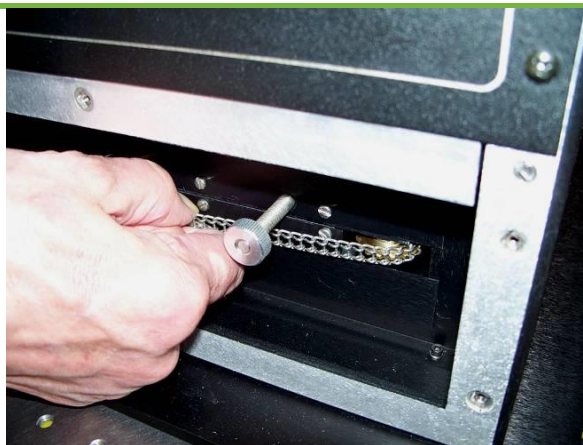
Figure 29: Adjustment using the ladder chain.
