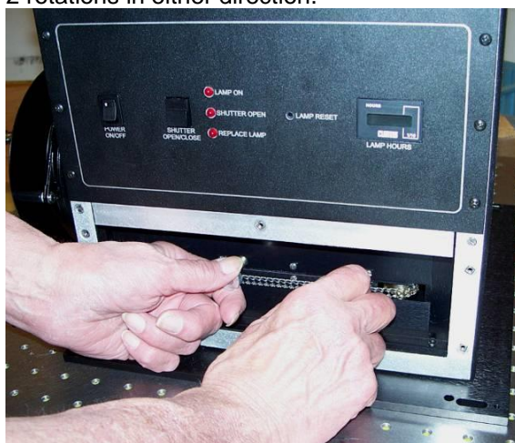
Figure 30: Adjustment using the X-Y knobs.
