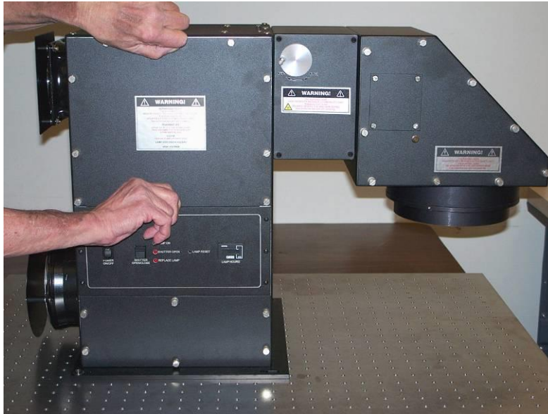
Figure 10: Removing the lamp access panel.
